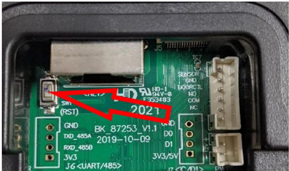
Fig.2. Factory reset – button on the plate
